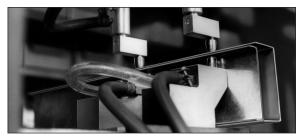
A Case Study: Dual spot welding of panelled wall sections reduced welding costs enough to justify buying welding machine to do the job in-plant. Equa-Press holder with 5-inch spacing, and special (but simple) tooling to provide two offset tip adapters and matching holders were used. Electrodes are standard TUFFCAP caps.
