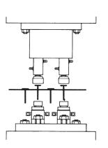
In this drawing, two studs are projection welded in each welder stroke, using an Equa-Press dual holder over a pair of studwelding electrodes held in PMstyle holders.
