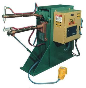
adjustable. Welder equipped with 2 1/2" diameter (2CR) or 2 3/4" diameter (3CR) copper horns and 1 1/4" diameter ejector type electrode holders using #2 M.T. water cooled electrodes. Unit comes complete with all necessary airline components, including: solenoid operated air valve, filter, regulator, gauge, lubricator and adjustable flow control valves. A shrouded foot switch is also supplied and interconnected.
