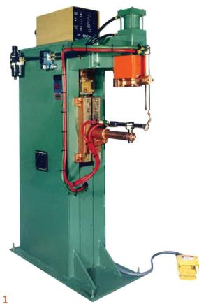
through side-mounted tap changer. Welder equipped with 2" diameter horns and ejector type electrode holders using #1 M.T. and water cooled electrodes. Unit comes complete with all necessary airline components including: solenoid valve, filter, regulator, lubricator and gauges. A shrouded, single stage foot switch is also supplied and interconnected.
