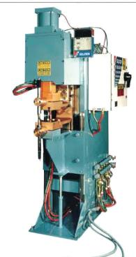
electrode holders. Stacked iron core transformer features water cooled cast copper secondaries for high production applications. Variable heat range selection, adjustable through side-mounted tap changer. Unit comes complete with all necessary airline components, including: solenoid valves, airline, filter, regulator, lubricator, gauge and flow control valves, all mounted for easy maintenance. A sturdy, shrouded foot switch is also supplied and interconnected.
