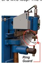
a limit switch when it moves downward a certain distance. At the start of each weld, the loop is sent downward before movement of the upper electrode. If the ring is stopped by a finger or other object before reaching the top of the part being welded, the limit switch does not trip and the electrode won't close.
