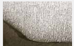
Nitrode after 1200 welds
