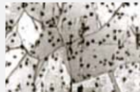
CuCrZr before and after annealing at 900°
